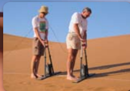
Nick Lancaster (right) and Geoff Duller (University of Aberystwyth) conduct high-resolution ground penetrating radar imaging of the internal sedimentary structure of a Namib Desert sand dune.
